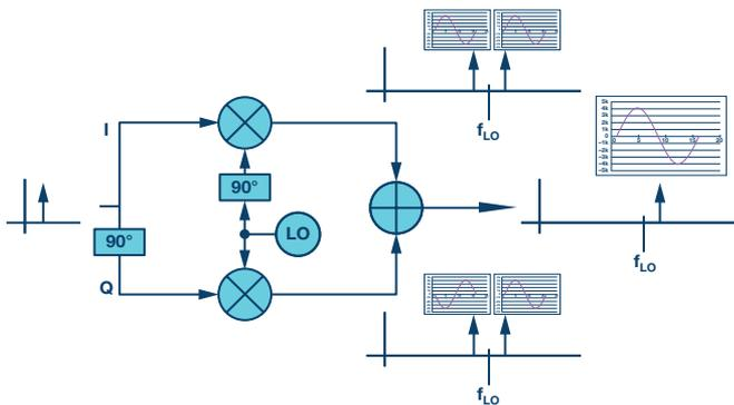
Figure 4. Simultaneous I and Q signal path analysis.
