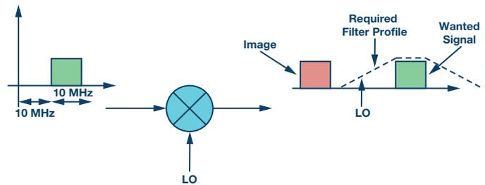
Figure 6. Single-mixer image filter requirements.
