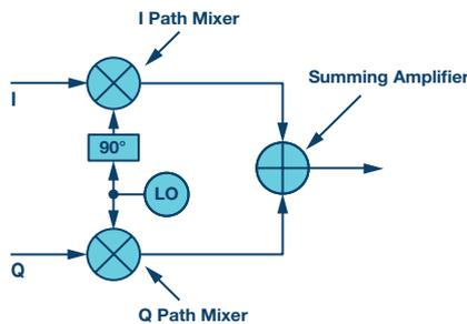
Figure 1. Basic architecture of a complex transmitter.
