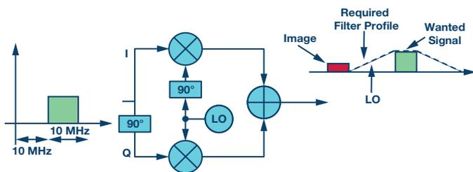
Figure 10. Practical implementation of the complex mixer. Note the attenuated image.
