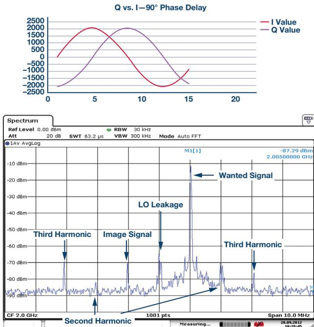
Figure 5. Tone placement dependent of the I and Q phase relationship.
