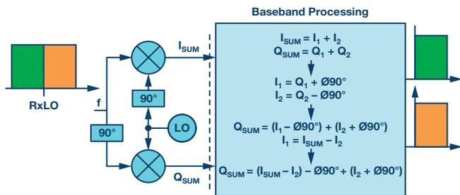
Figure 9. Zero-IF complex mixer receiver configuration.
