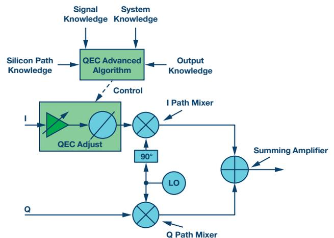
Figure 12. Advanced QEC algorithm and smart silicon design enabling zero-IF architecture.
