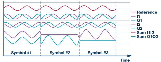
Figure 8. Taking a closer look at I/Q signaling in a zero-IF complex mixer configuration.
