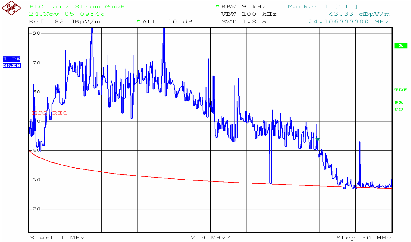
Figure 2: Radio spectrum emitted by PLC installation (measured in open area in a distance of 3 m from power supply line carrying PLC signals). Spikes are intended radio signals emitted by licensed radio transmitters. The line on the bottom presents the limits according to CEPT ECC/REC/(05)04).
